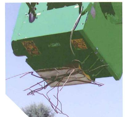
Montabert's crusher buckets offer a new approach to **processing and recycling stone**, asphalt and concrete debris **on-site**. These tough buckets can eliminate the expense of separate crushing and handling equipment, and make **costly dumping** and transport **unnecessary**. An electromagnetic iron-separating magnet is optional, and easily installed on-site.
