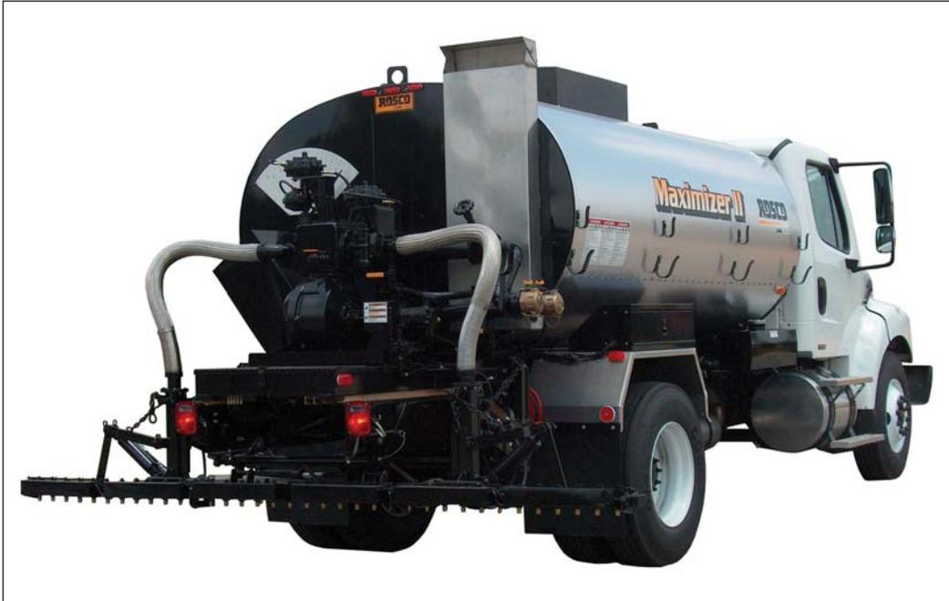
*Rosco's Maximizer II asphalt distributor puts the operator in full control from the clean, safe comfort of the cab. Maximizer II's Plus-1 controller controls application rate and spray width in 1-foot sections while on the move. The Viking asphalt pump and clog-free spraybar valves make Maximizer II a reliable workhorse on the job. Clean-up is a snap with the Enviro-Flush clean out system.*
