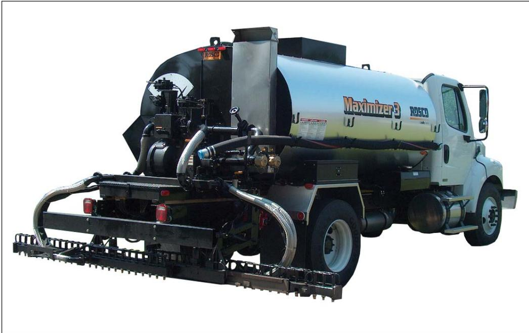
*Rosco's Maximizer 3 asphalt distributor features an extendible spraybar that smoothly moves from an 8-foot to 16-foot width in 4-inch increments. The EZ-Spray extendible spraybar makes radius and taper spraying, along with maneuvering for obstacles such as bridges, a smooth and efficient operation.*
