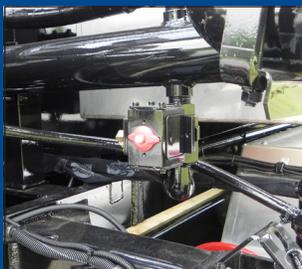
**1** Activate Enviro-Flush Cleanout Cycle. Automated valve opens and adds a small amount of solvent to the system.
