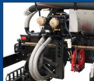
**3** Reopen Enviro-Flush valve and reverse pump to return solvent to 25-gallon tank to be reused again and again.
